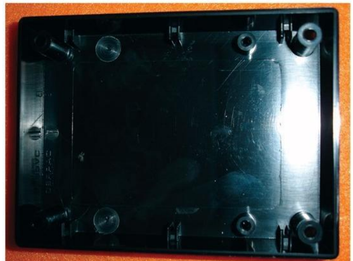
■ FIGURE 3. Milled out posts.
